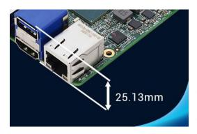
Measuring just 85mm x 56mm, the <u>UP 710S</u> was an excellent option for discrete deployment within the robotic arm's space-constrained housing. Further, the board's layout was designed with the CPU on the I/O-side, resulting in a 10mm height reduction,
