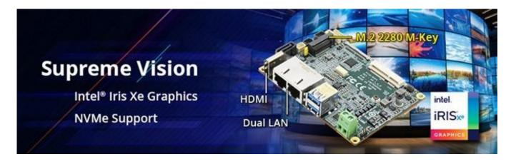
The <u>PICO-RAP4's</u> FPC connector allowed for MIPI camera integration, along with two high-definition cameras connected via its USB 3.2 Gen 2 ports to capture multiple sources of visual data, supported by Intel® UHD Graphics. Additionally, the board's two serial ports provided RS-232/422/485 signal interfaces for connecting GPS modules and environmental sensors.
