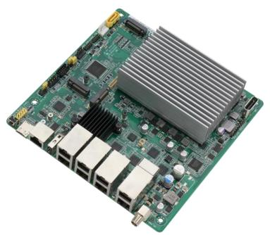
Upon review, the customer felt that a product from AAEON's Mini-ITX motherboard range, the MIX-ASLD1, would be the most suitable option. For practical reasons, the board was secured in custom housing, providing access to the necessary interfaces for its role as an IoT Gateway while protecting it from dust ingress and
