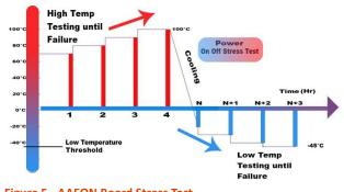
Figure 5 - AAEON Board Stress Test
