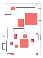
Figure 2 - Poor Thermal Component Design
