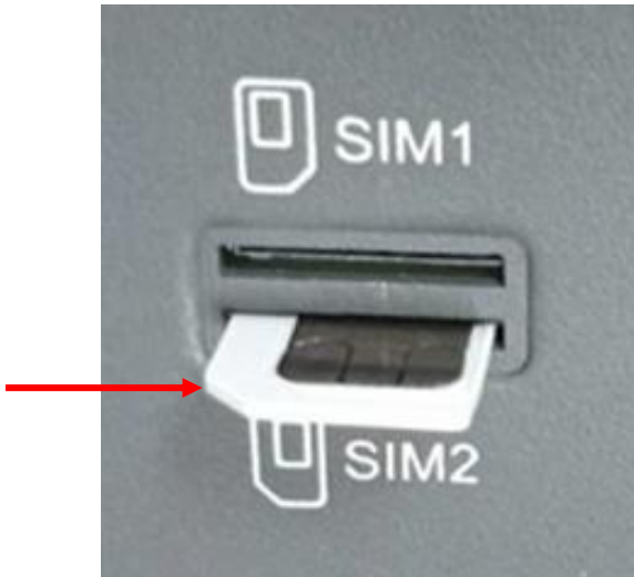
SIM 2: Exposed card side up, notch is facing to the left.
