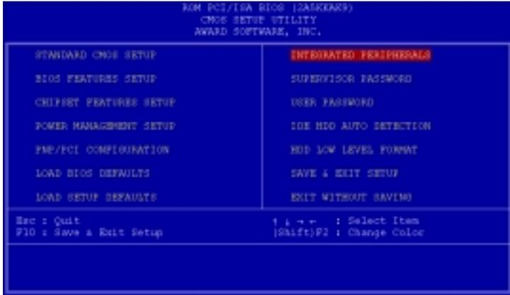
By choosing the INTEGRATED PERIPHERALS option from the initial SETUP SCREEN menu, the screen below is displayed.
