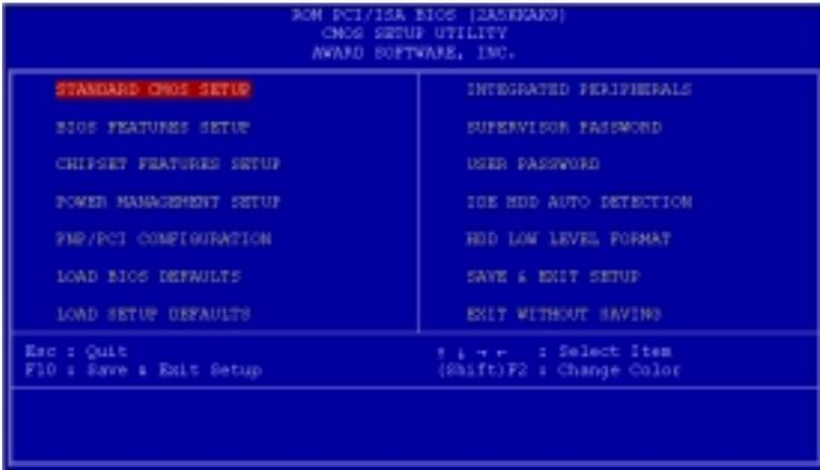
When you choose the STANDARD CMOS SETUP option from the INITIAL SETUP SCREEN menu, the screen below is displayed.
