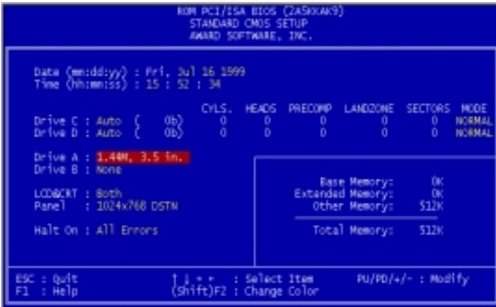
This standard setup menu allows users to configure system components such as the date, time, hard disk drive, floppy drive, display, and memory. Online help for each field can be accessed by pressing F1.
