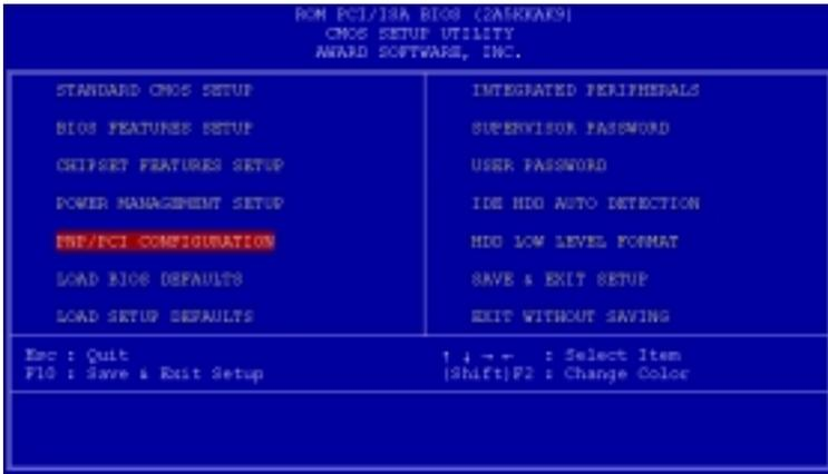
By choosing the PNP/PCI CONFIGURATION SETUP option from the initial SETUP SCREEN menu, the screen below is displayed.
