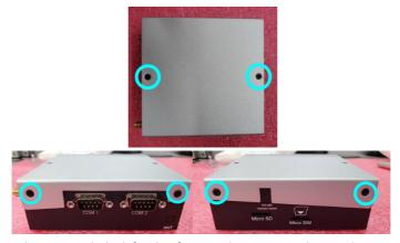
Step 2: Open the antenna hole (left side of system) by removing the punch-out cover.
