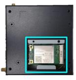
**Step 5:** Connect the antenna cable to the module.
