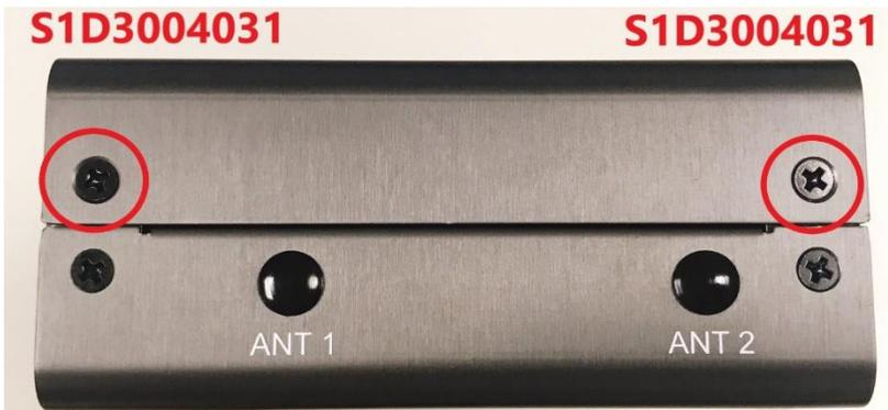
**Step 2:** Next, remove the two screws securing the cover on the top:
