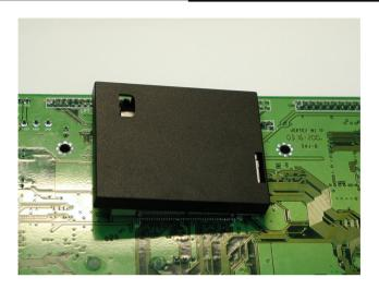
Step 4: Press a little bit with the finger on the hole of the cover.
