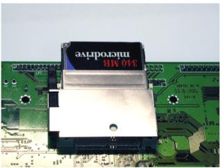
Step 2: Push the CompactFlash Card forward until the end.
