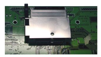
Step 3: Put the cover on from the right to left and hook up the CompactFlash Card white base with the crook on the cover.
