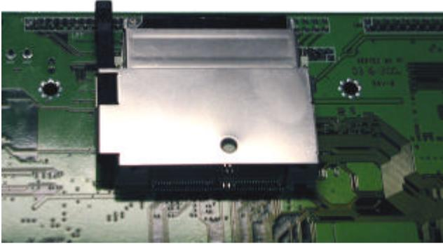
**Step 3: Put the cover on from the right to left and hook up the CompactFlash Card white base with the crook on the cover.**
