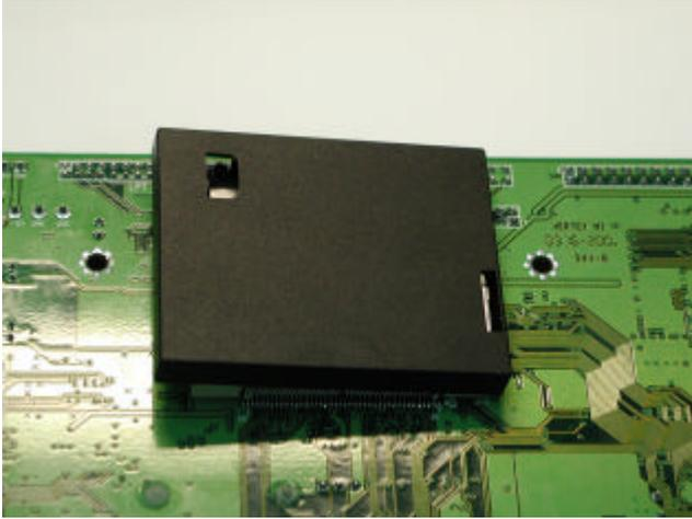
**Step 4: Press a little bit with the finger on the hole of the cover.**
