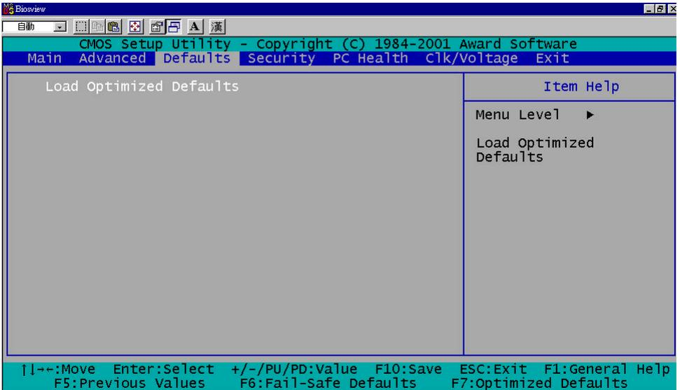
Pressing "Y" loads the default values that are manufacturer's settings for optimal performance system operations.
