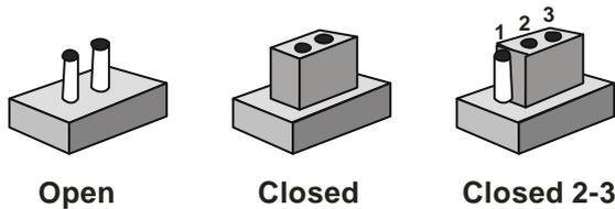
A pair of needle-nose pliers may be helpful when working with jumpers.
