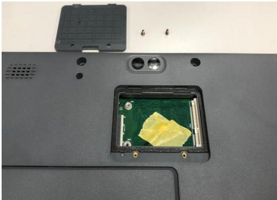
3. Remove the tape and pull up the antenna cable
