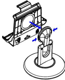
2. Press and hold clips inward and insert the holding plate through the circular hole, release the clips to secure
