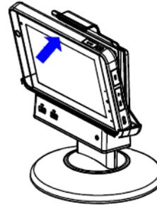
3. Place the RTC base-first onto the plate, push back to secure
