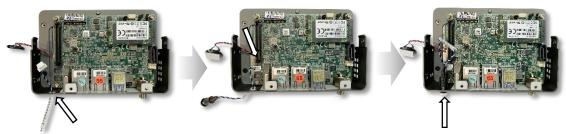
**Step 10:** Peel the backing off of the tape on the CMOS battery. Gently press the battery onto the PICO-KBU4 board to secure it.
