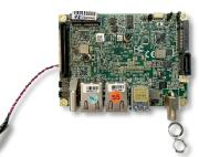
**Step 4:** On the processor side of the PICO-KBU4 board, install the memory RAM module. Insert at an angle (~30°) and then gently press down until it is secured in place.
