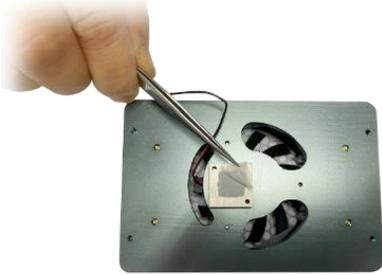
**Step 2:** Place the top chassis onto the thermal assembly. Note the orientation of the chassis with the thermal assembly. Secure with four black screws.
