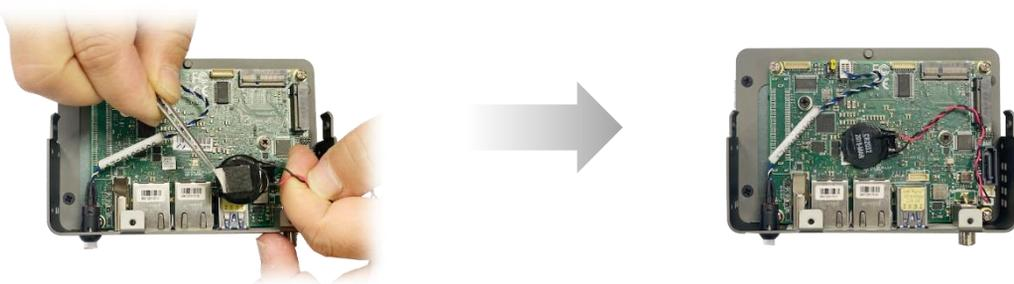
**Step 9:** Attach the bottom chassis by first lining up the right side, then swivel the chassis into place. NOTE: the bottom chassis does not slide directly on, it must swivel into place as shown in the figure.
