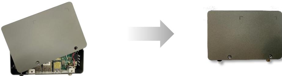
**Step 10:** Ensure the bottom chassis is properly lined up and attached. Use black screws to secure, two screws on the bottom and one screw on the left and right sides of the chassis.
