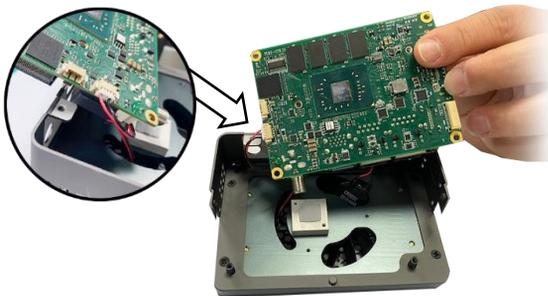
**Step 5:** Insert the PICO-APL4 board into the chassis assembly with the processor side toward the thermal assembly. DO NOT place the CMOS battery between the board and thermal assembly.
