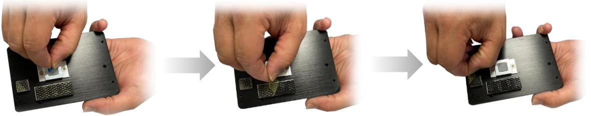
**Step 2:** Place the top chassis onto the heatsink. Note the orientation of the chassis with the heatsink. Secure with four black screws.
