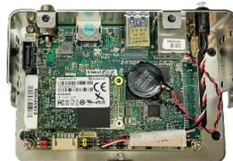
**Step 11:** Attach the bottom chassis by first lining up the right side, then swivel the chassis into place. NOTE: the bottom chassis does not slide directly on, it must swivel into place as shown in the figure.
