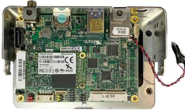
**Step 8:** Check that the I/O ports are properly aligned. Secure board with four nickel screws.
