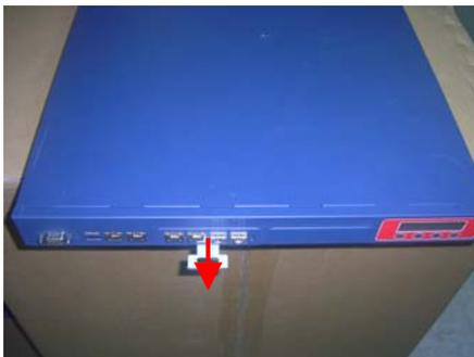
Step 3: Insert the LAN Module and fasten the screw
