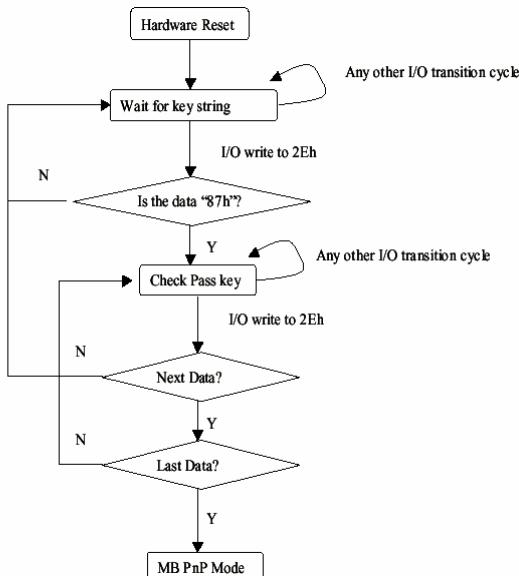
There are three steps to complete the configuration setup: (1) Enter the MB PnP Mode; (2) Modify the data of configuration registers; (3)
