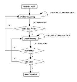
There are three steps to complete the configuration setup: (1) Enter the MB PnP Mode; (2) Modify the data of configuration registers; (3) Exit the MB PnP Mode. Undesired result may occur if the MB PnP Mode is not exited normally.
