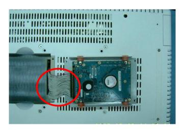
5. Fasten the four screws on rear side to lock the HDD bracket
