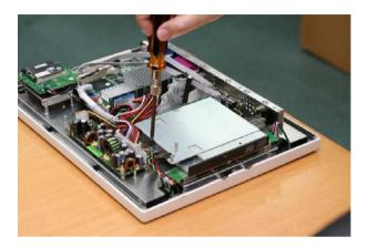
9. Fasten the two screws to lock the speaker
