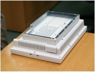
4. Fix the rack with the screws on the corners.
