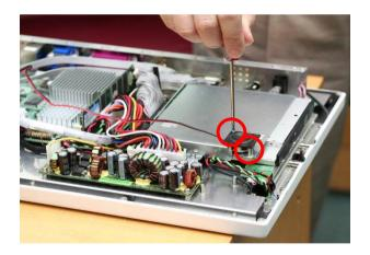
Lock the plastic cover of the ONYX-150 and complete the installation
