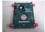
Adhere sponge on HDD bracket and place HDD into bracket
