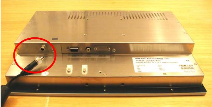
A "Surge Protection" device plugged between the AC-DC adapter and the wall outlet is recommended to prevent the effects of sudden current variations from reaching the LCD monitor. The sudden peaks of electricity may harm the LCD monitor.
