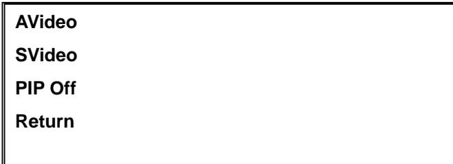
Picture-in-picture enable function allows you to view screen with VGA input and A-Video or S-Video sources at same time. Use up and down arrows to select major viewing source. Press Menu to enter your selection. The second input source window will be displayed on the bottom right corner.
