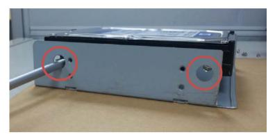
Step 5: Fasten six screws on the each side of bracket to 3.5" and 2.5" HDD cases (Upper one is 3.5"HDD and lower one is 2.5" HDD, total 12 screws)
