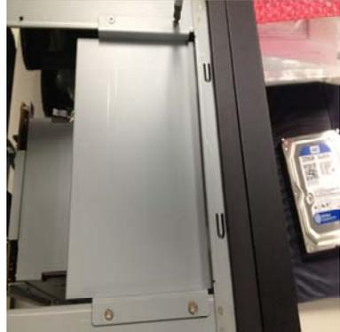
Step 2: Shift the HDD upper bracket from right to left and remove it.
