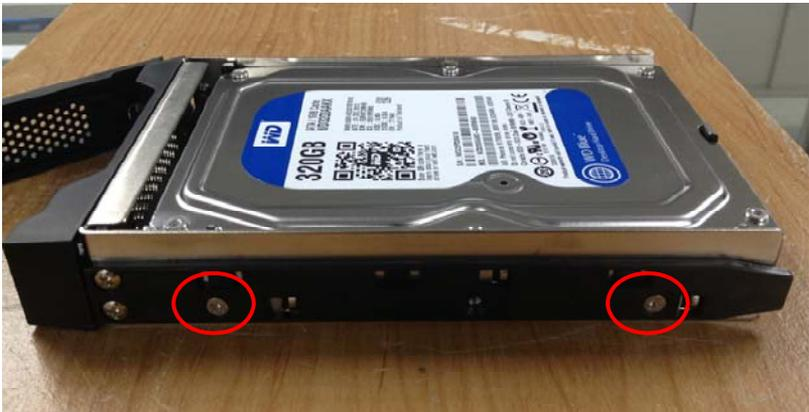
Step 5: Put the HDD into the bay.
