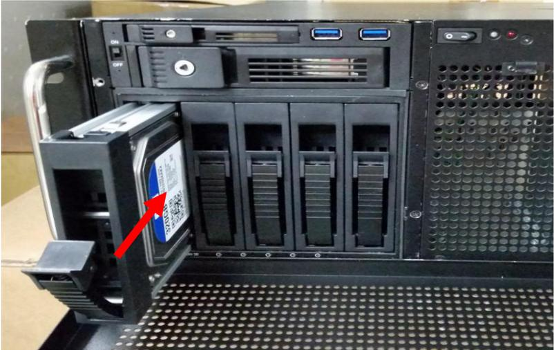
Step 4: Push the lever to latch the HDD tray
