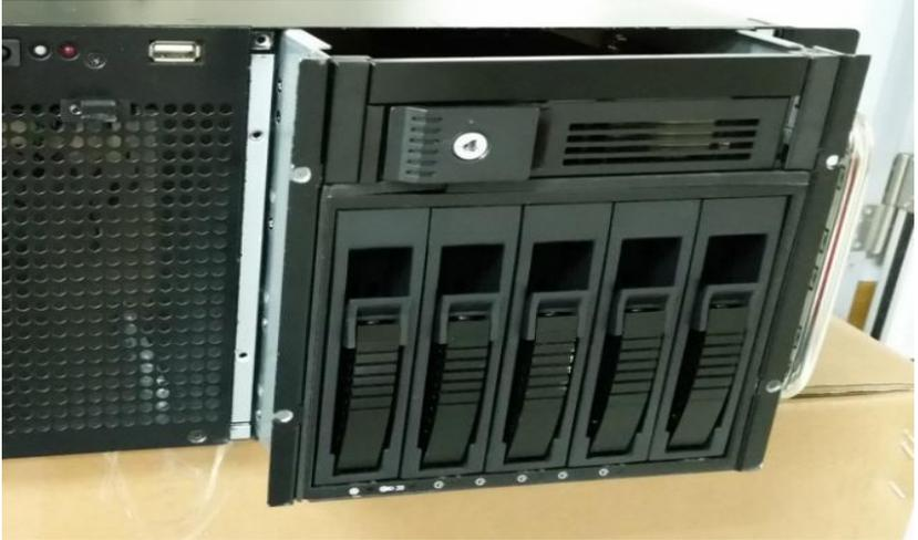
Step 4: Remove the slim optical drive bay by pressing buttons on both sides
