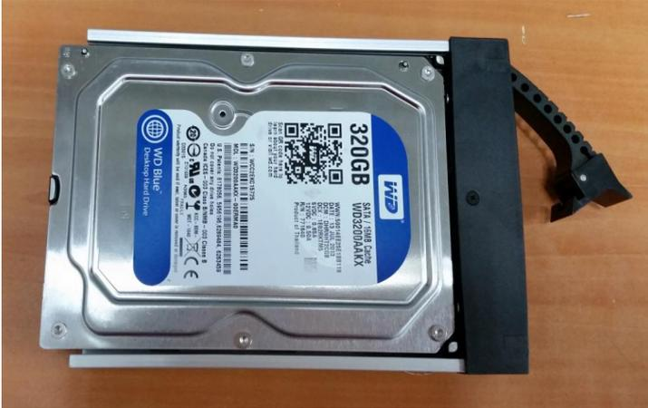
Step 2: Fasten the four screws to secure the HDD with the HDD tray
