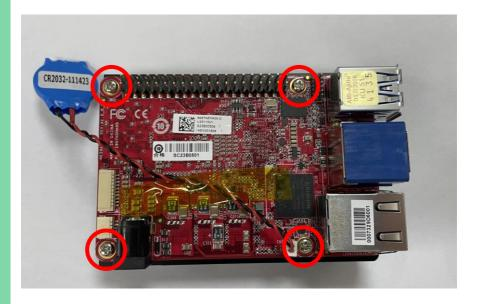
Step 2: Affix and lock the four (4) pillars to the board in the following sequence.
