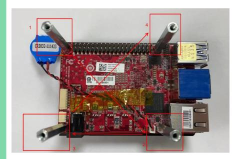
Affix and lock the four (4) pillars from heatsink side.
