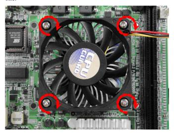
Notice that when you are locking it, you need to fasten it with the strength that exerted on four screws balancedly. If you fasten it with the strength on one single screws alone and keep it extremely tight, it may cause the process to the damage.
