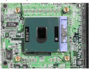
Step 1: Put the processor on the socket
