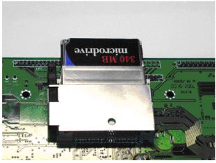
Step 2: Push the CompactFlash Card forward until the end.
