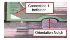
Step 3: (Positioning the CPU into socket)
