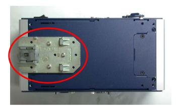
Step 2: Press the DIN Rail on the DIN Rail kit to fix it.
