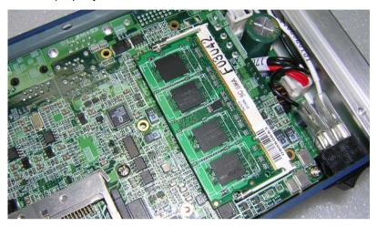
Step 6: Adhere the heat-spreading sheet to the SDRAM
