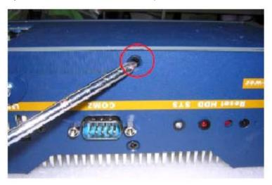
Step 2: Loose the screw on the rear panel of AEC-6822
