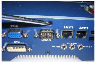
**Step 3:** Unfasten the four screws on the bottom case of AEC-6822
