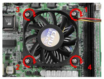
Notice that when you are locking it, you need to fasten it with the strength that exerted on four screws balancedly. If you fasten it with the strength on one single screws alone and keep it extremely tight, it may cause the process to the damage. We strongly suggest you to fasten the four screws in order. (From the screw 1 to screw 4 showed above.)
