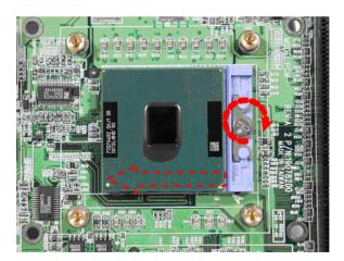
When you turn the screw rightward, the socket will move to left then steady lock the processor.
