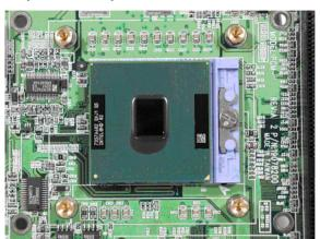
Step 1: Put the processor on the socket
