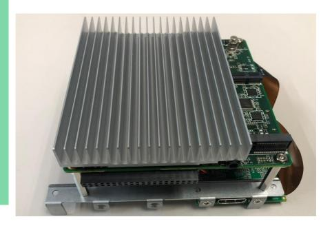
**Step 1**: Affix and lock the four (4) screws and the four (4) pillars (28mm) to the board in the following sequence.
