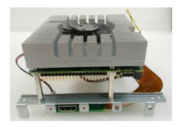
Step 1: Remove the two (2) screws from the outer edges of the board.
