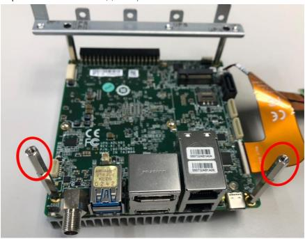
Step 7: Affix and lock the two (2) sliver screws to the HDMI IN carrier board.
