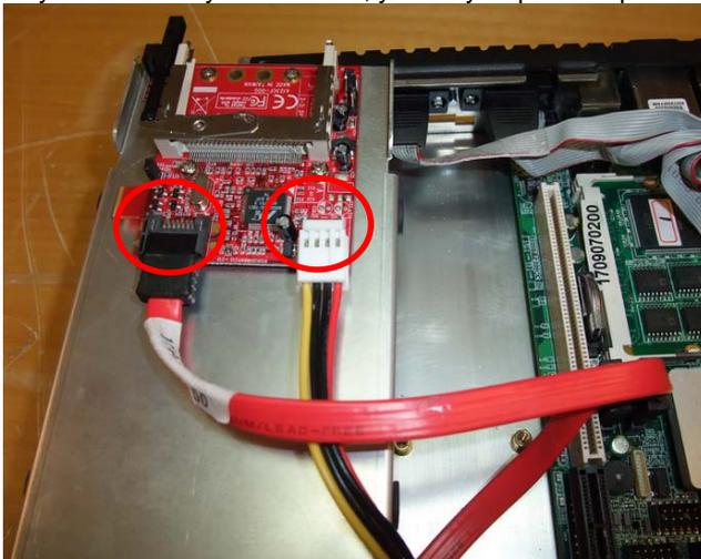
Step 4: Unfasten the four screws to release the CompactFlash Card
