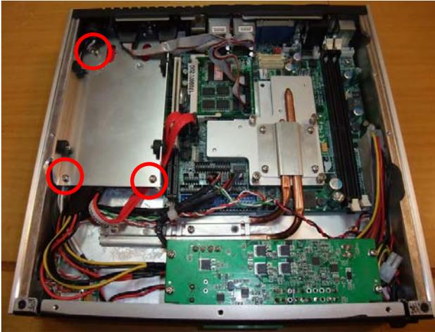
Step 3: Disconnect the SATA and Power cables (The CompactFlash card is optional. If you did not buy the CF card, you may skip the step 3 and step 4.)
