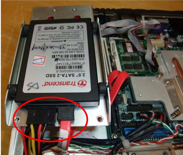
Step 8: Place the HDD case to the GES-3300F and press the case to insert the HDD to the GES-3300F
