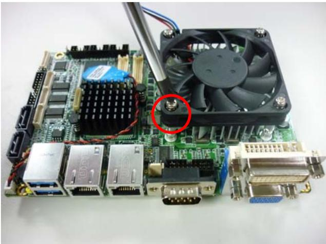
Step 3 : Fasten the screw at the right-up side
