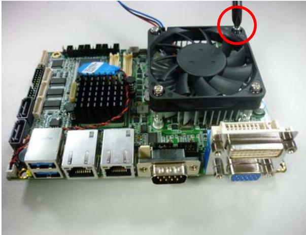
Step 4 : Fasten the screw at the right-down side
