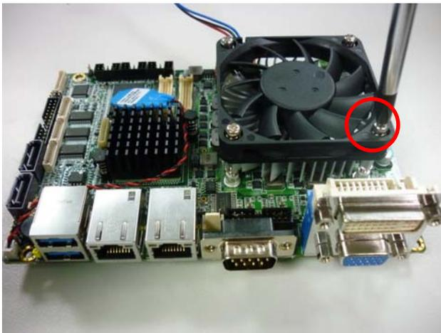
Step 5 : Fasten the screw at the left-up side as the picture
