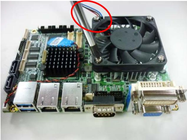
Step 2: Fasten the screw at the left-down side first
