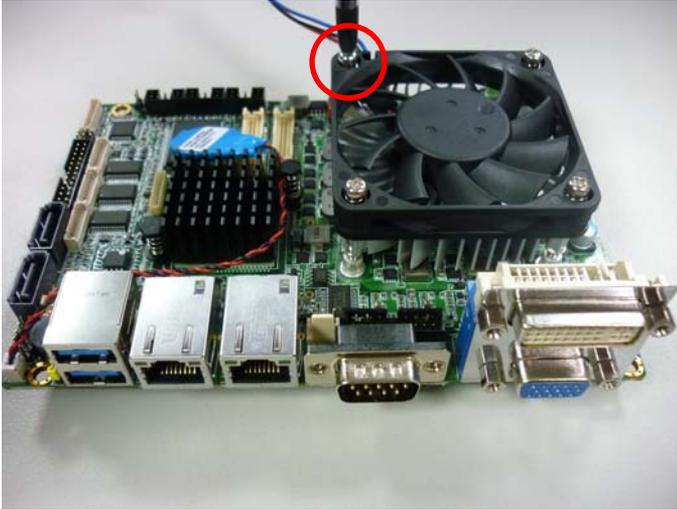
Step 6 : Connect the Fan Cable to the Fan Connector
