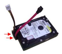
**Step 3:** Fasten the Serial-ATA hard disk drive to the firewall board from the bottom of the chassis with four screws.
