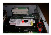
Step 4: Insert the Mini PCI Card obliquely.
