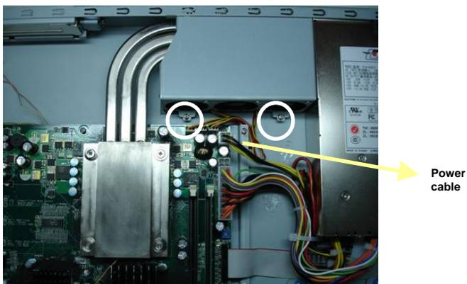
Step 15: Insert the Power cable of Fan Module
