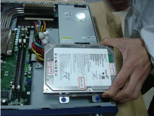
Step 5: Fasten the four screws of the Hard Disk Drive Bracket
