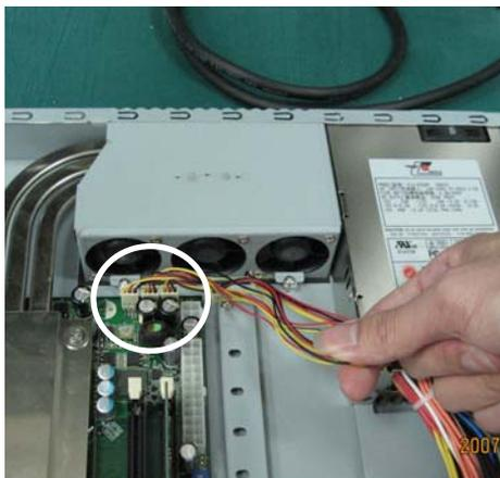
Step 3: Loosen these two screws and pull off the power cable of the three fans
