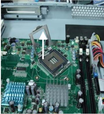
Step 6: Put the CPU on socket
