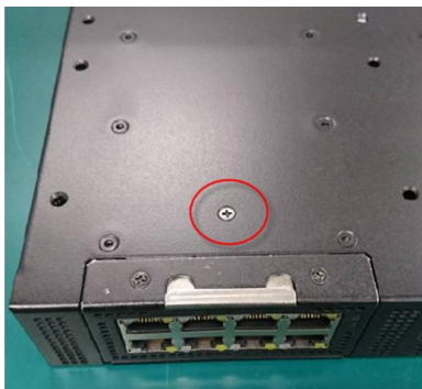
Replacing NIM Module
