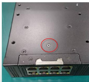
Replacing NIM Module
