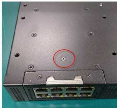
2. Remove the null module cover or existing module.
