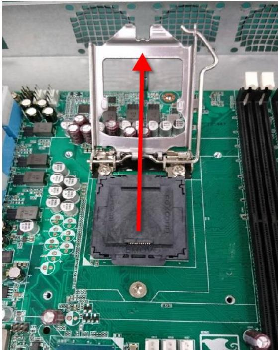
3. Remove the cover and place the CPU into the socket. Make sure the two fillisters are properly locked.
