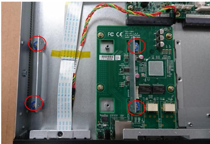
3. Place the HDDs into the bracket, tighten the screws to secure
