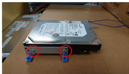
4. Place the assembled HDDs back into the system, secure with screws and reattach the SATA and power cables.
