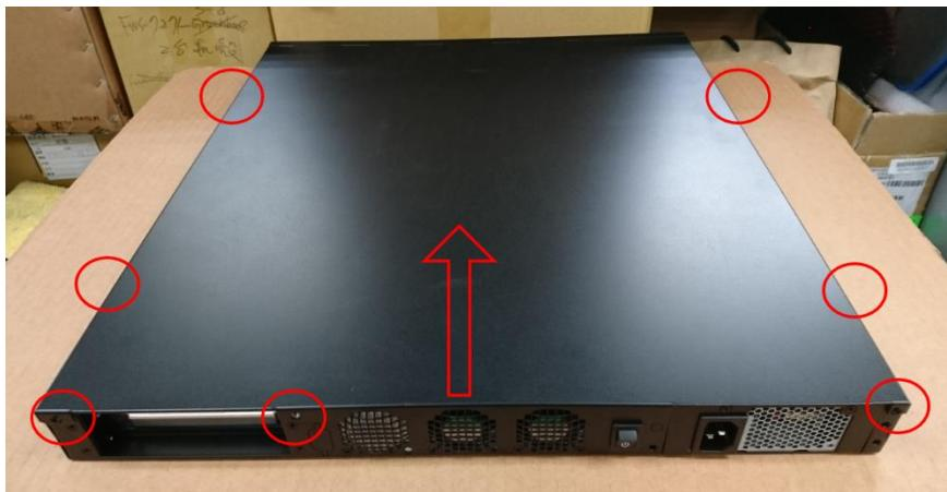
2. Remove the screw to remove the cover bracket
