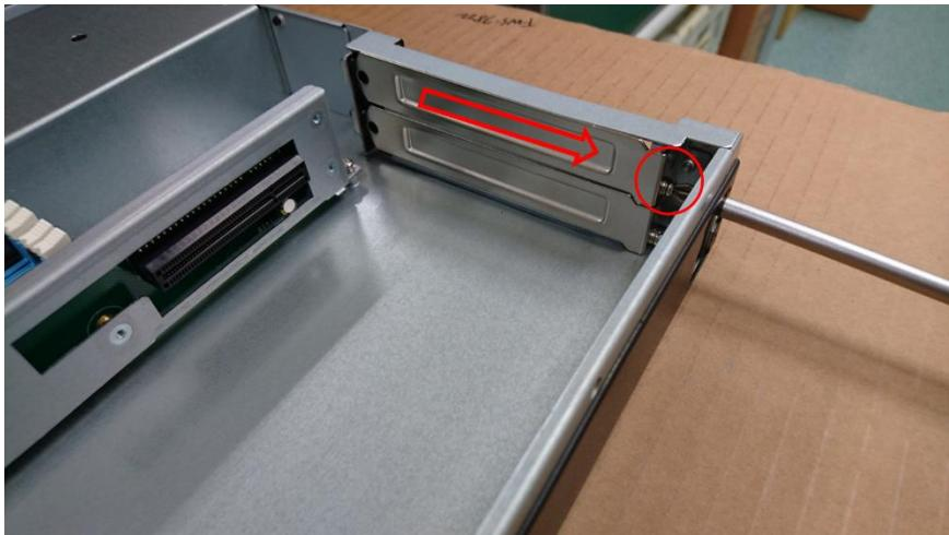
3. Firmly insert the expansion card into the slot and secure the screw.
