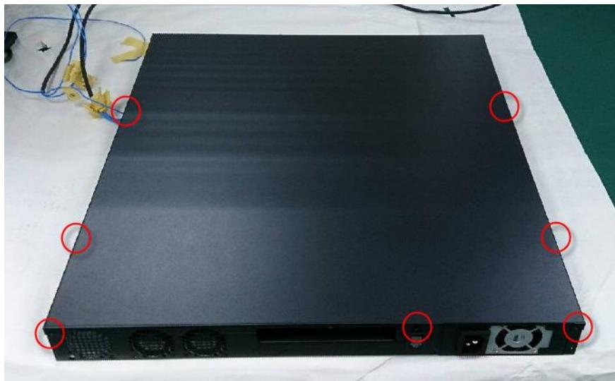
2. From the front of the system, slide it upwards to remove
