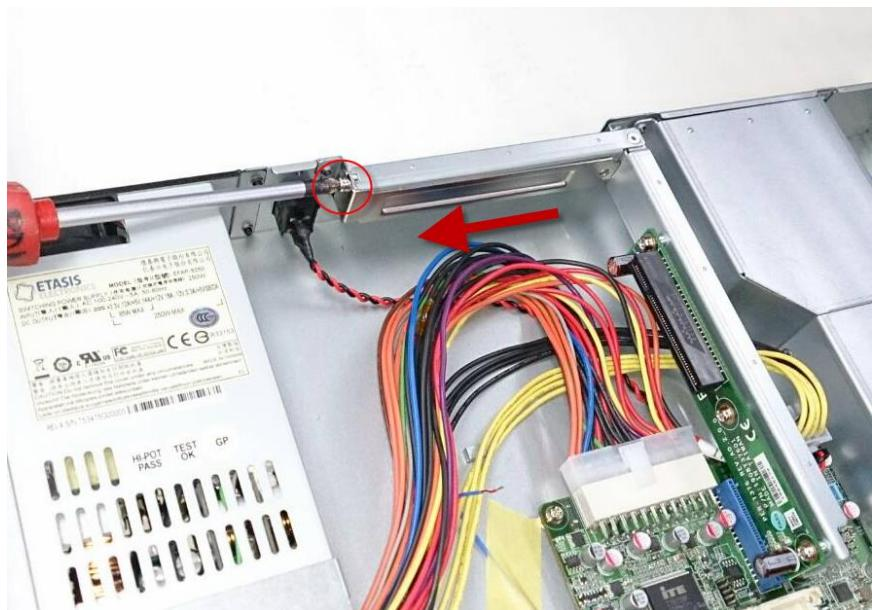
4. Firmly insert the expansion card into the slot and secure the screw.
