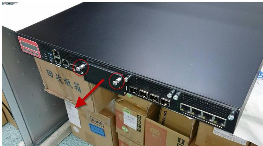
2. Remove the highlighted screws to remove the NIM
