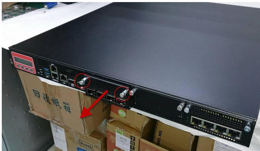
3. Insert the NIM and secure with screws
