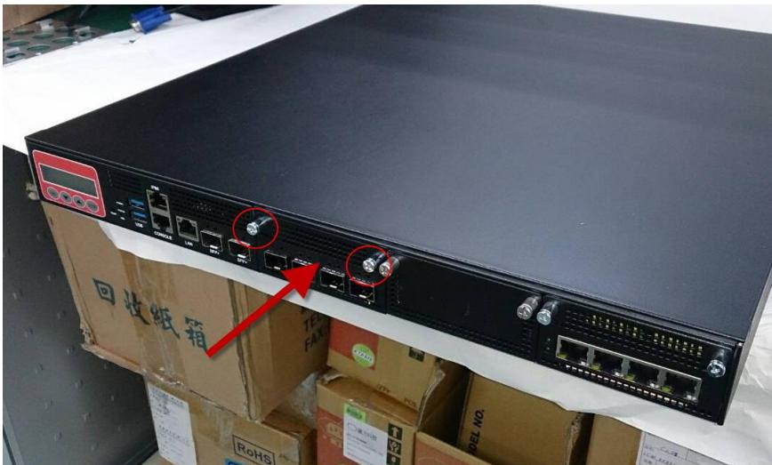
4. Close the NIM cover and secure with screws
