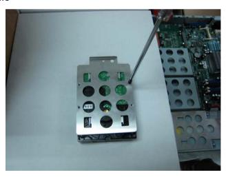
Step 4: Lift down the hard disk drive and push into the bracket
