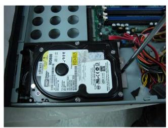
Step 6: Connect the SATA cable and power cable into the Hard Disk
