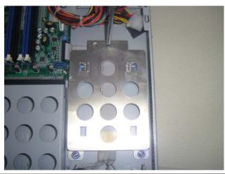
Step 2: Lift up the hard disk drive bracket aside
