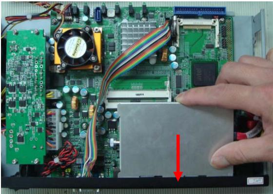
Step 6: Lock the HDD case horizontally
