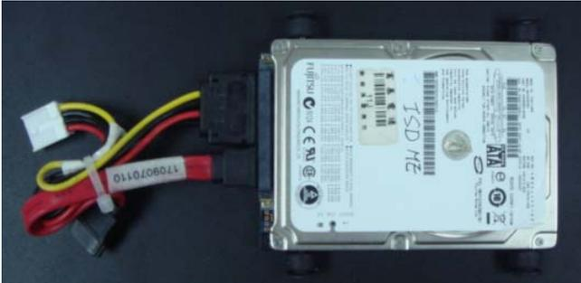
Step 4: Place the HDD to the HDD Case that got from the chassis and make sure four rubber feet have been wedged in the flutes
