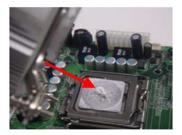
Fasten the four screws. First fasten the two screws (yellow) and then fasten the two screws (red) in sequence to secure the heatsink in place.
