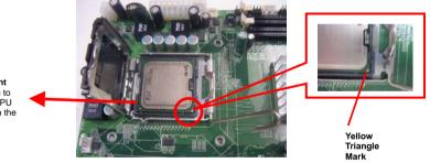
The **Alignment Key** is for you to check if the CPU is aligned with the CPU notch properly.  Close the upper plate (A), place the load lever back to the original position and tightly wedge the lever into the fastening tab. (B)
