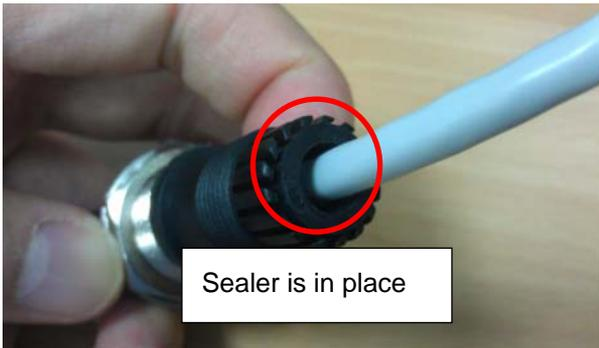
Step 8: Before locking the plastic rear nut tightly, press the cable hardly and make sure all parts of the LAN connector has been connected tightly
