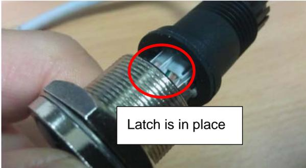
Step 6: Lock and tighten the nut of RJ-45 plug
