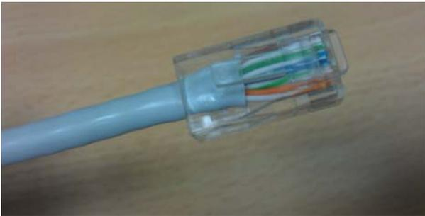
Step 5: Insert RJ-45 plug into the socket and mount to cable set's body. Make sure the latch of RJ-45 connector is in place
