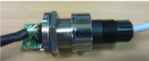
Step 7: Screw on the plastic rear nut a little bit for locking later.
