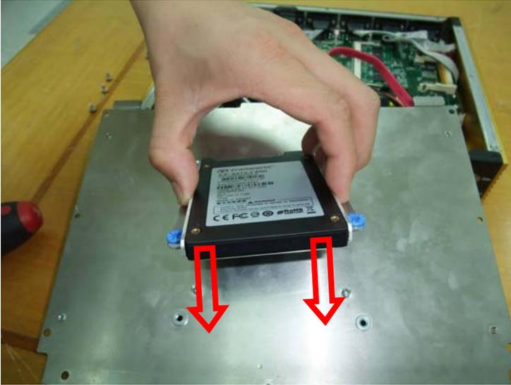
Step 6 : Fasten 4 screws on bottom case.
