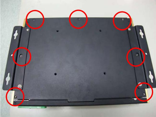
Step2 : Move bottom case from FES-5130, the four screws at bottom case will be fastened by HDD tray.
