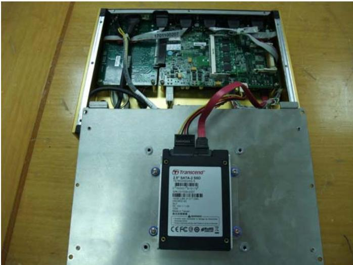
Step 9 : Fasten the seven screws on the bottom case of FES-5130.
