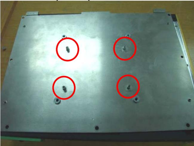
Step 3 : Fasten four screws on HDD Tray.
