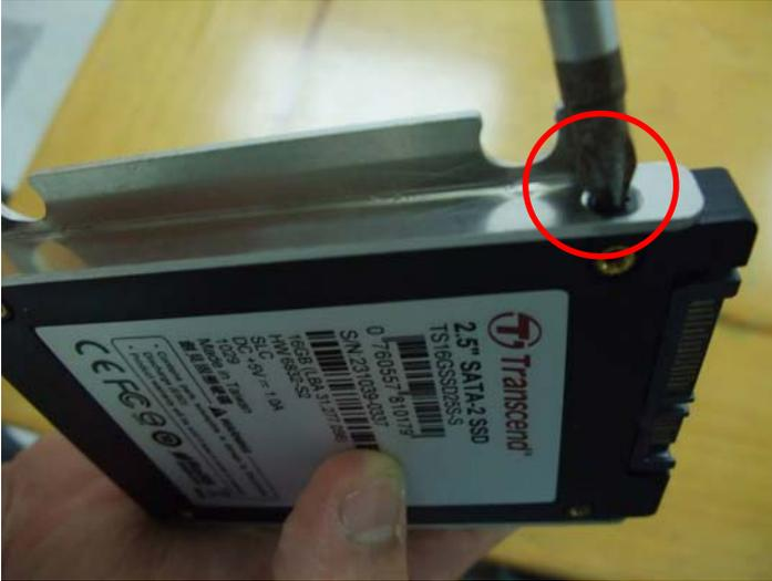
Step 4 : Put plastic rubber damper of anti-vibration on HDD tray.
