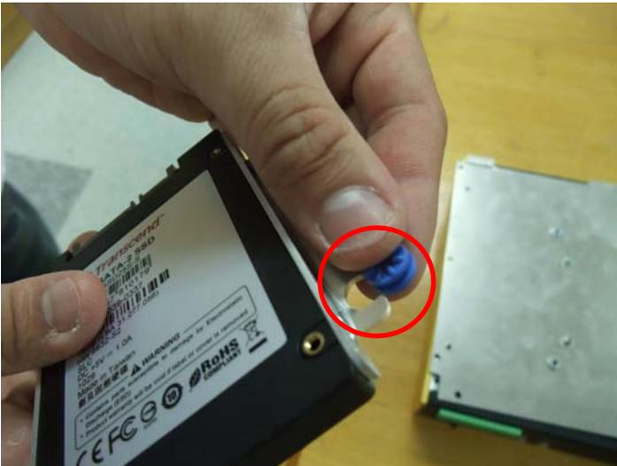
Step 5 : Put HDD with Tray on bottom case.
