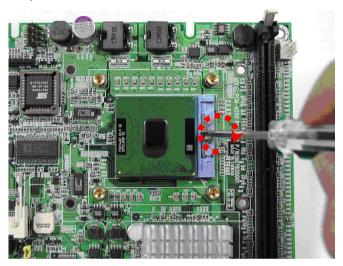
When you turn the screw clockwise, the socket will move to left and lock the processor.
