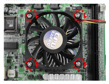
Note: when you are locking the cooler, please fasten the four screws with the equal strength to prevent the processor from damage.
