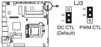
EMB-Q87A Inverter Backlight Control mode selection
