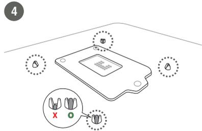
To uninstall the CPU heatsink and fan assembly
