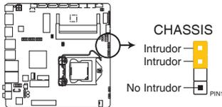
**EMB-Q87A Chassis intrusion connector**
