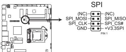
**EMB-Q87A SPI flash programmable connector**
