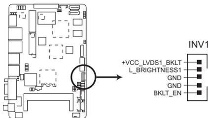
**EPC-CV1 Backlight inverter power connector**
