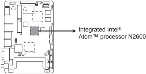
**EPC-CV1 Integrated Intel® Atom™ processor N2600**
