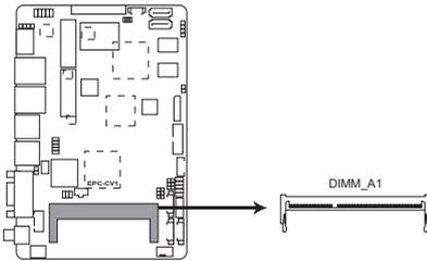
**EPC-CV1 DDR3 DIMM socket**
