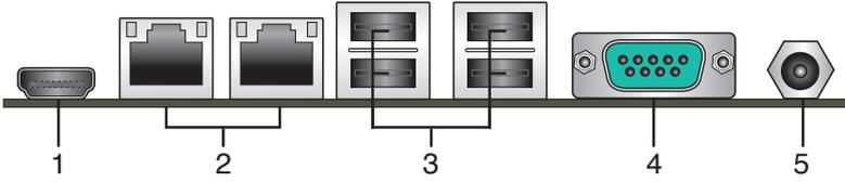
1. **HDMI port.** This port is for a High-Definition Multimedia Interface (HDMI) connector, and is HDCP compliant allowing playback of HD DVD, Blu-Ray, and other protected content.
