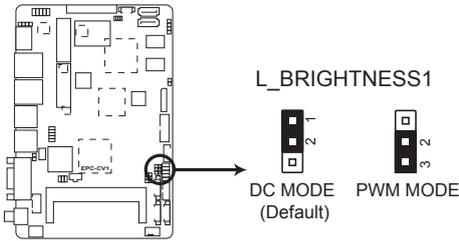
**EPC-CV1 LVDS backlight brightness control jumper**
