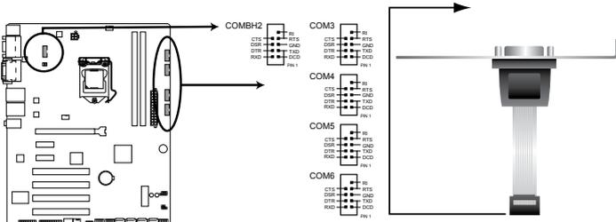
**IBM-H61A Serial port connectors**
