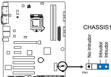
**IMBM-H61A Chassis intrusion connector**
