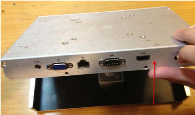
Step 5: Loosen the Hard Disk Drive (HDD) bracket on the standoff with two screws
