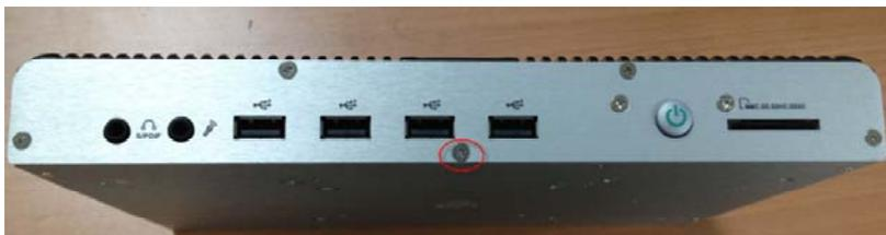
Step 3: Unfasten the four screws on the rear panel
