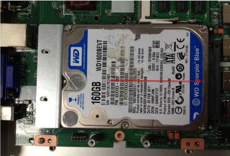
Step 9: Lock the bracket of HDD on the standoff with two screws
