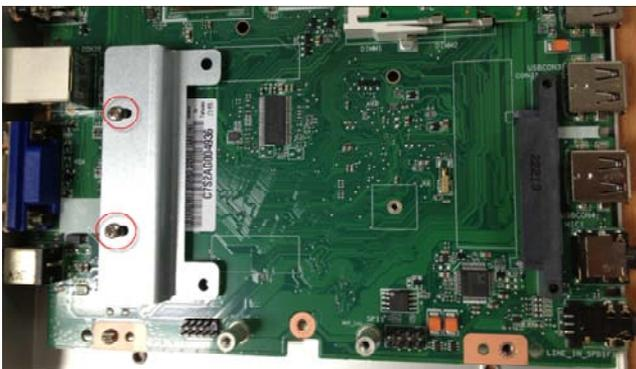
Step 6: Lock HDD on the HDD bracket with two screws
