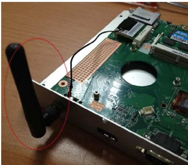
Step 4: Install the Wi-Fi module and fix it by a screw
