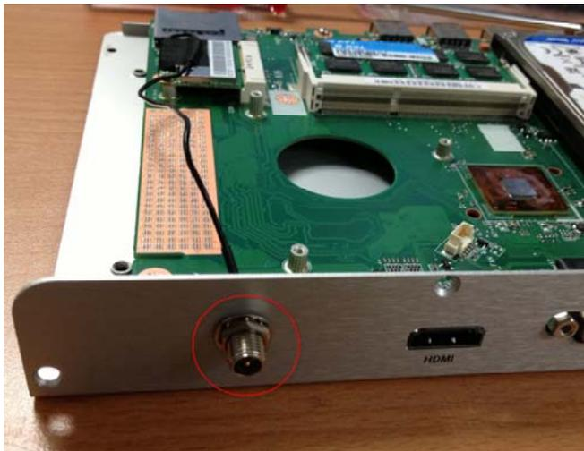
Step 3: Screw the antenna on the connector
