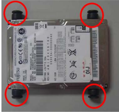
Step 5: Put the HDD to the HDD case and close the upper bracket of the HDD case. Make sure the damper are locked by the flutes on the bracket
