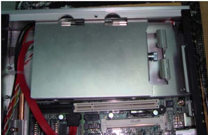
Step 3: Pull out the knob and turn the knob left or right at a 90-degree angle to open the HDD case
