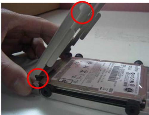
Step 6: Turn the knob left or right at a 90-degree angle conversely and the knob will recoil to the case automatically to lock the HDD case
