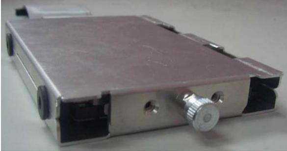
Step 7: Insert the HDD case to the DSS-5300 horizontally and lock the HDD case
